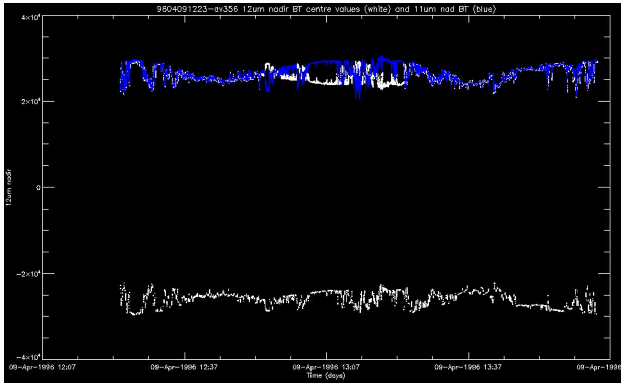
Figure 2: Brightness temperature values from (approximately) the centre of scan for orbit at 12:23 09-Apr-1996. 12µm values in white, 11µm in blue. The lower white trace with negative values is caused by blanking pulse flags in the data.
