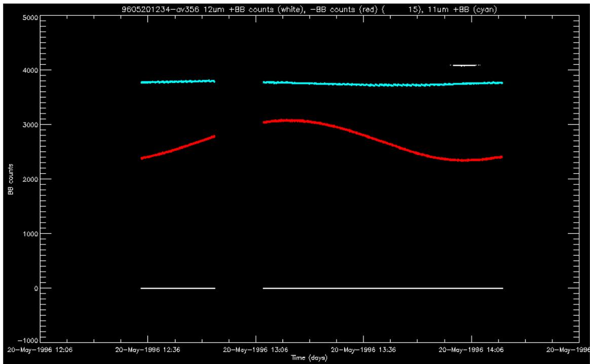
Figure 17: Counts from the 12µm channel warm (white) and cold (red) blackbodies and from the 11µm channel warm blackbody, for the orbit at 12:34 20-May-1996
