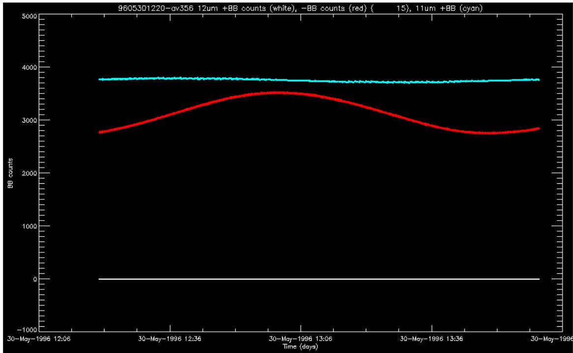
Figure 18: Counts from the 12 $\mu$ m channel warm (white) and cold (red) blackbodies and from the 11 $\mu$ m channel warm blackbody, for the orbit at 12:20 30-May-1996
