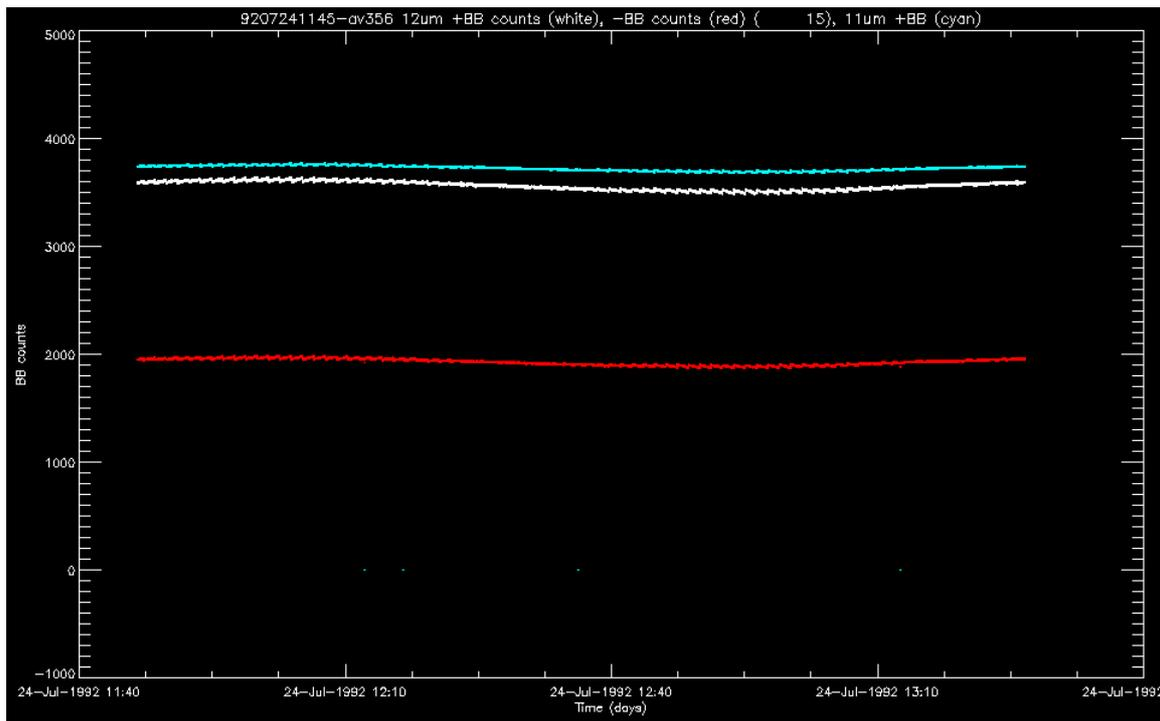
Figure 5: Blackbody counts from the 12µm channel warm (white) and cold (red) blackbodies and from the 11µm channel warm blackbody, for the orbit from 24-Jul-1992 11:45.
