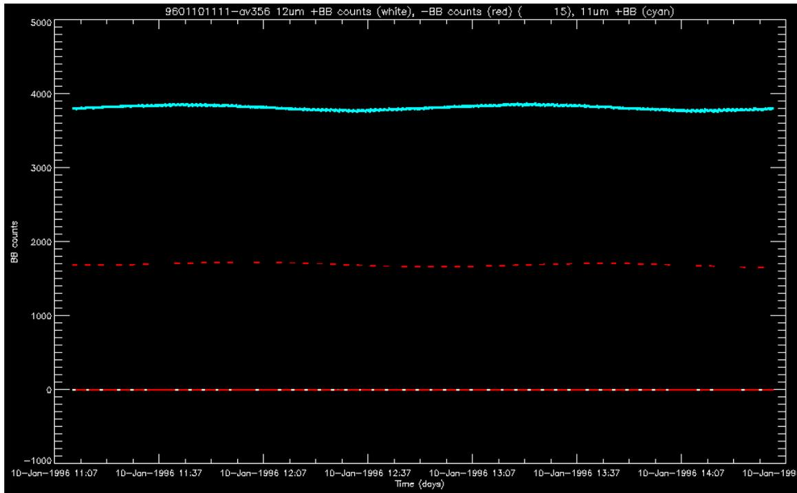
Figure 10: Counts from the 12µm channel warm (white) and cold (red) blackbodies and from the 11µm channel warm blackbody, for the orbit at 1996-01-10 11:11
