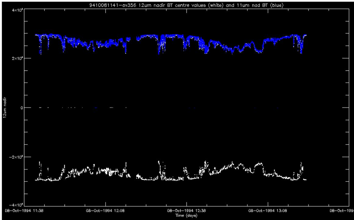
Figure 8: Brightness temperature values from (approximately) the centre of scan for orbit at 11:41 08-Oct-1994. 12µm values in white, 11µm in blue.
