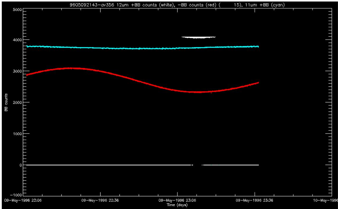
Figure 14: Counts from the 12 $\mu$ m channel warm (white) and cold (red) blackbodies and from the 11 $\mu$ m channel warm blackbody, for the orbit at 21:43 09-May-1996
