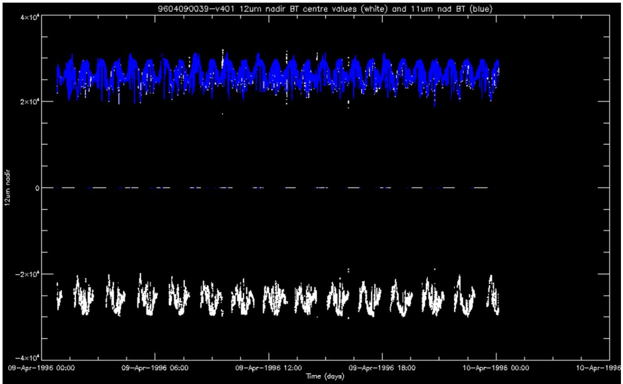
Figure 23: Centre of scan brightness temperatures for the whole day of 09-Apr-1996, 12µm and 11µm channels, from the updated SUPPLE processor.
