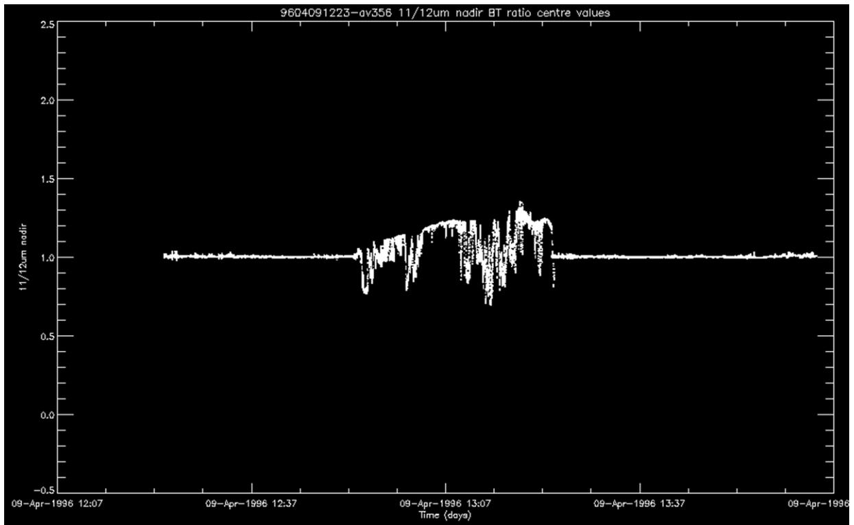
Figure 3: Ratio of the centre-scan brightness temperatures in the 11 $\mu$ m and 12 $\mu$ m channels, for the orbit from 09-Apr-1996 12:23.
