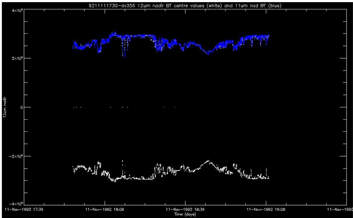
Figure 7: Brightness temperature values from (approximately) the centre of scan for orbit at 17:30 11-Nov-1992. 12µm values in white, 11µm in blue.
