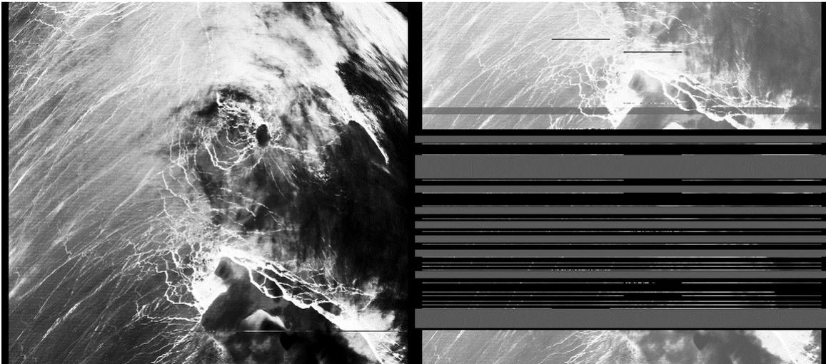
Figure 29: 11µm nadir scene 9604091042-09736 from Level 0 version 9120 (left) and version 8700 (right). In version 8700-derived UBTs the feature near the centre of the scene is shifted into the next product, which has along-track distance 09985, only 249 different from the preceding scene rather than the usual 512.
